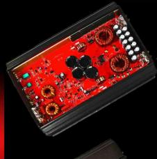
Ultra Efficient Class D topology reaching 83% efficiencies at full power, provides the biggest power in the smallest chassis. SMT assembly and 1% resistors round out a proven Power-House for any subwoofer system. 67,200 mfd capacitance on the battery inputs and 25,000 mfd capacitance on the outputs reinforcing the seat of the pants feeling that you can only get from a MMats Amplifier. Leading many people to say "MMATS amplifiers are extremely underated".
